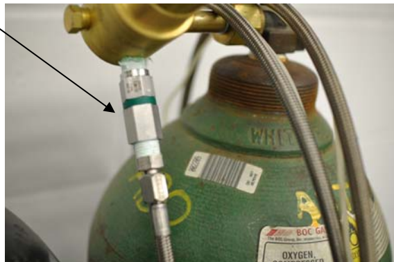
Excessive Flow Valve (Included with 2013 Models. Factory Recommended for Retrofit on 2005 Models)
